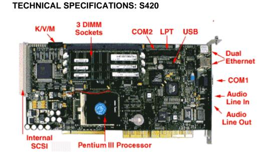
For projects requiring high server density and Pentium III performance with 133MHz front-side bus and memory expansion to 1.5GB, Cubix offers the S420 server. The S420 also features a sound chip for those applications requiring audio support.
